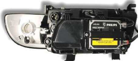
XENON headlight with nverter
